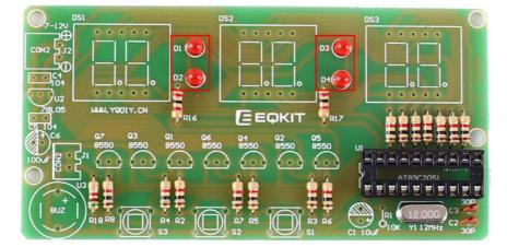
Step 8:Install 2pcs 0.1uF Ceramic Capacitor at C4,C5.
